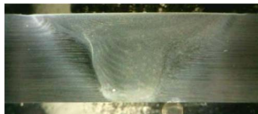
Fig. 4: Macrostructure of butt welded FSW joint. (Joon et al. [22])
