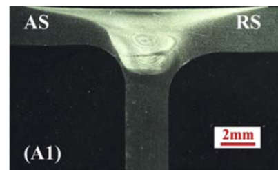
Fig. 8: Macrostructure view of T-joint configuration. (Yong Zhao et al. [32])
